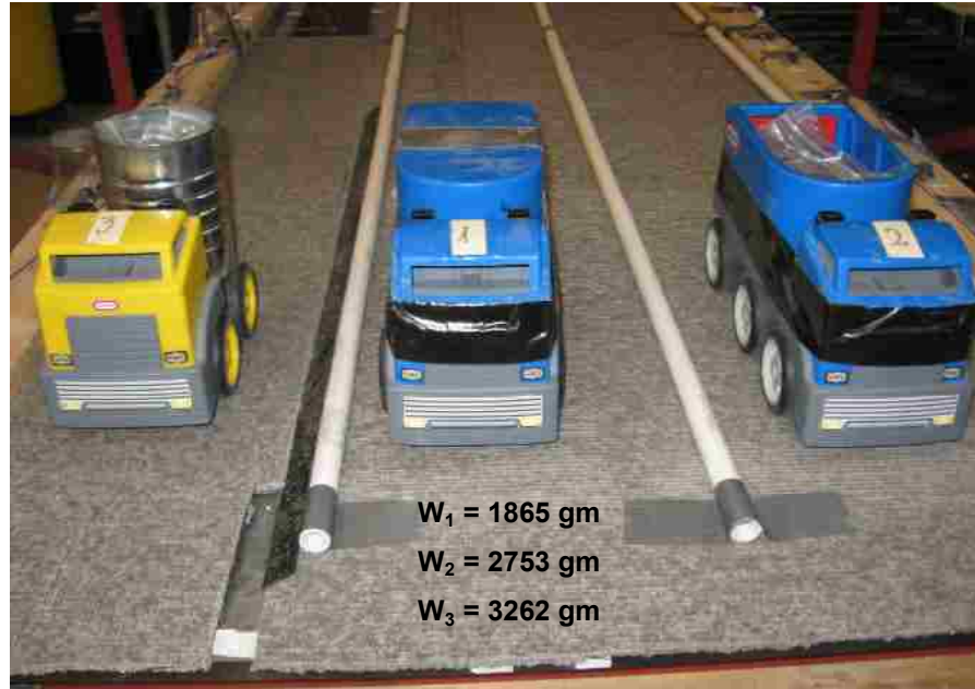
Figure 5-35 Model trucks with their weights.
