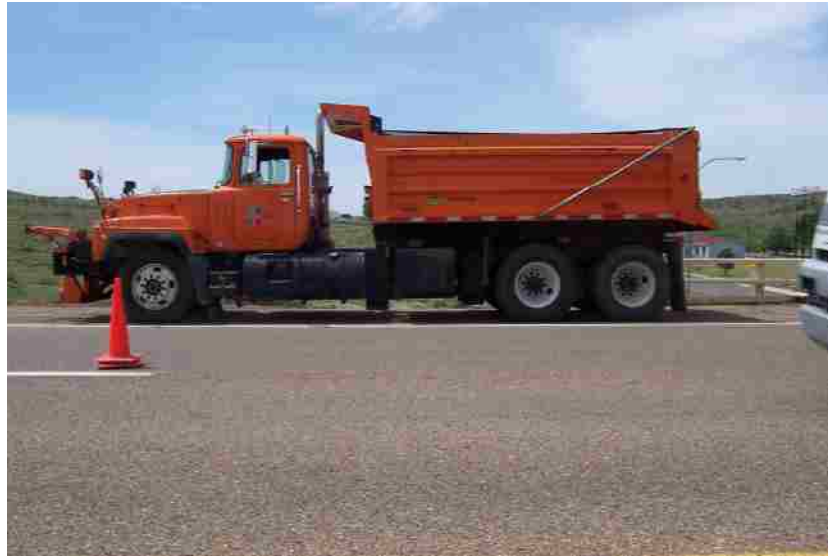
Figure 5-17 Mack 10 yard dump truck as test truck with weight of 50 Kips. Truck weight was determined at the day of field test.
